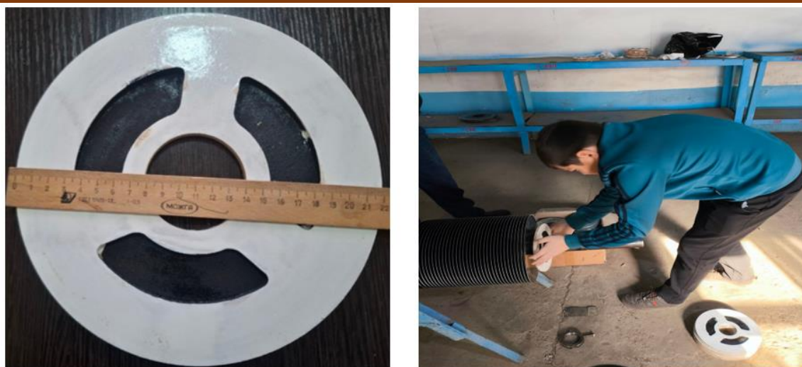
Figure 3 – Scenes from the process of assembling the prepared saw spacers into the saw cylinder
